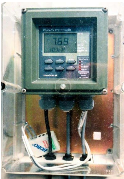
pH meter: An example of an automated pH meter linked to a system which treats the water to maintain a predetermined pH
