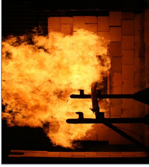
ISO 22899-1 Jet Fire test – before, during and after – Lloyds Register witnessed
