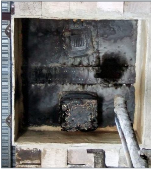
ISO 22899-1 Jet Fire test – before, during and after – Lloyds Register witnessed
