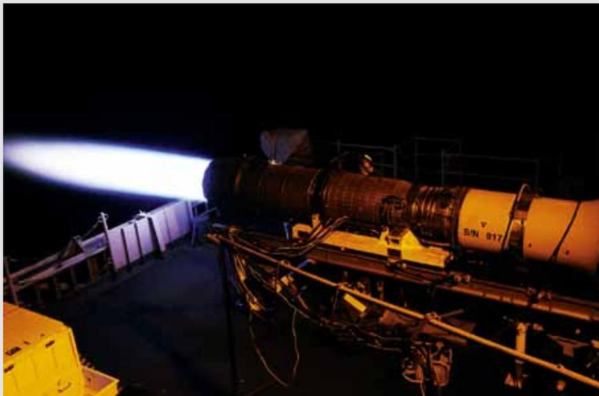
*Figure 2.* A U.S. sailor assigned to the aviation intermediate maintenance department's jet shop watches during a jet engine test cell on an F404-GE-400 jet engine for an F/A-18C Hornet aircraft on the fantail of aircraft carrier *USS Nimitz* (CVN 68), October 14, 2009, in the Indian Ocean. The F404 engine has twice won the Department of Defense Performance-Based Logistics Award. U.S. Navy photo by MC3 John Phillip Wagner Jr.
