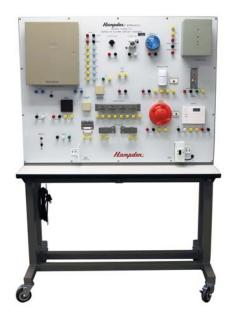
MODEL H-BACT-3 Dimensions (including mobile frame): 75"H x 48"W x 30"D Shipping Weight: 530 Lbs. The 1Ø branch circuit includes: single-pole Quicklag GFCI circuit breaker; adjustable load for ground fault insertion; AC milliammeter for monitoring ground fault current; and load connections consisting of output jacks and a duplex receptacle.
