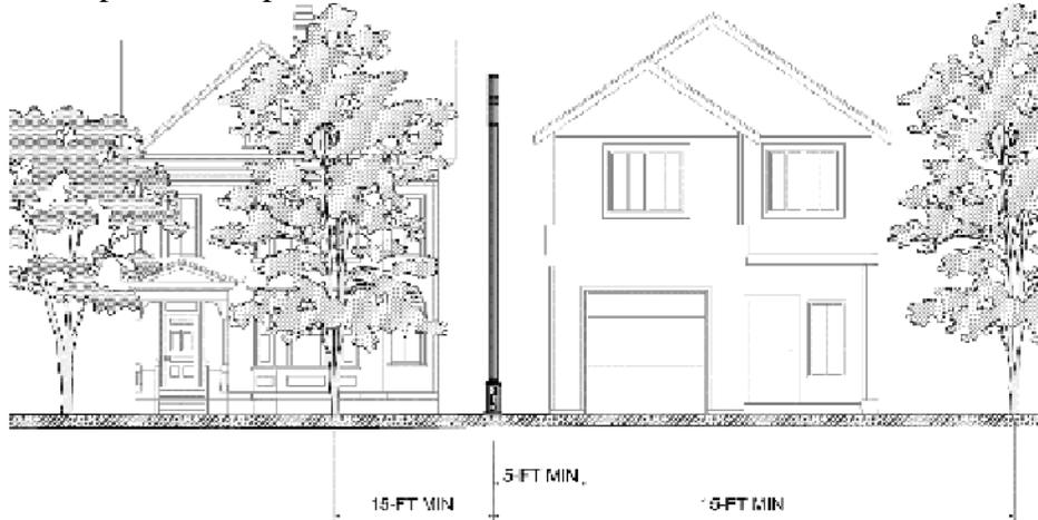
Figure 4-2: Example of Acceptable Location Between Commercial Buildings
