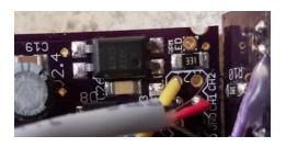
On V2.4 Pin labeled RPM LED (far right lower next to the resistor with the numbers 331 on top, not pictured) Give it a ground signal and it will pick up RPM. 1 pulse per cyl fire.
