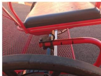
Springs on axel and on seat
