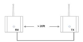
Note: The Rx and TX units should be separated by >20ft for optimal performance. An optional 50ft RJ11 patch cable (p/n: MP-52RJ11UNNE-050) is available if needed.
