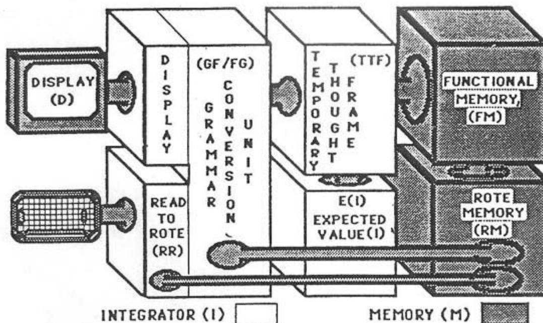
**READ TO ROTE (RR)** This is the keyboard unit into which all data is typed. The only real function of this unit is to transmit that which it receives to Rote Memory (RM).
