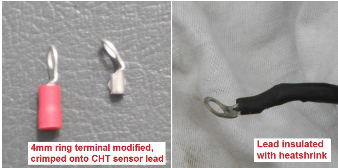
Figure 3 – CHT End Fitting
