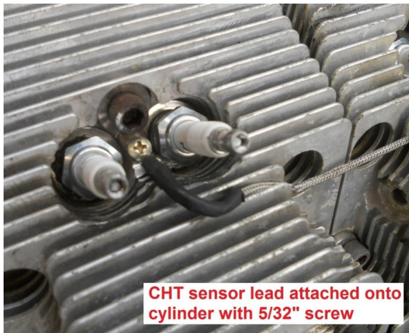
Figure 4 – CHT Cable Routing
