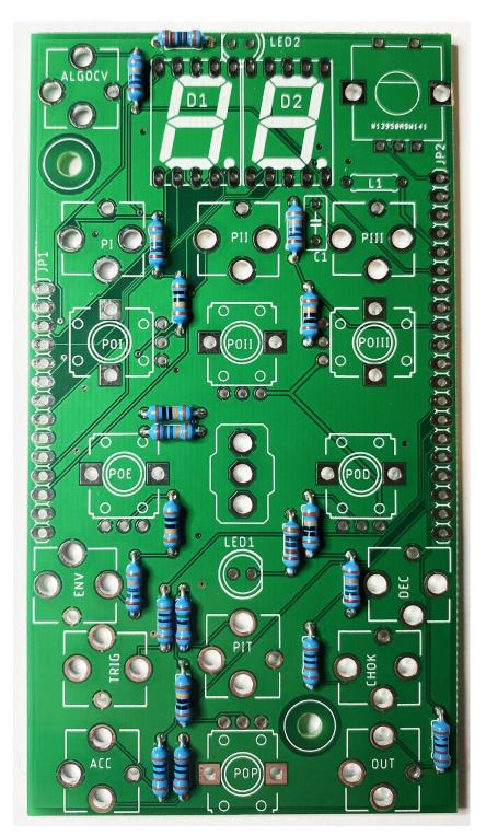
Install and solder C1 and L1
