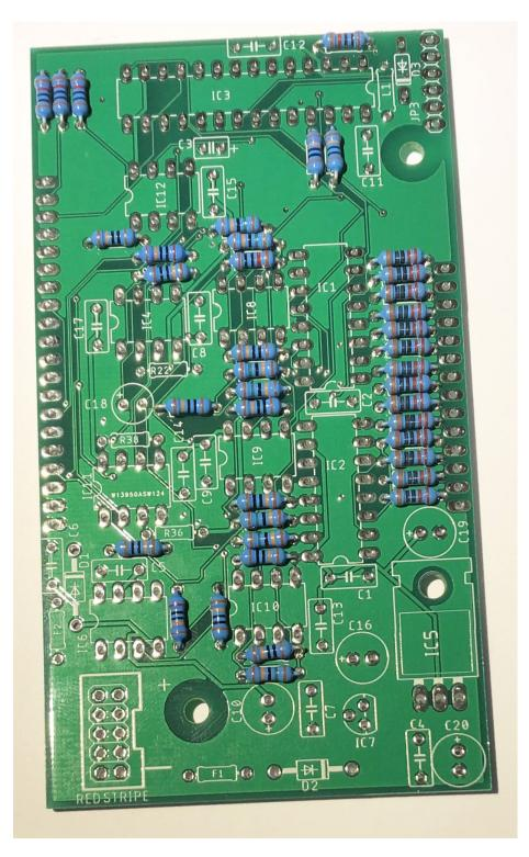
Install and solder the 300K resistor R36
