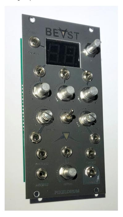
When everything is level and sitting nicely, flip it over and solder the remaining joints for the switch, jacks, pots. Maneuver the LED so it aligns up with the transparent parts of the panel as closely as possible and solder in place.
