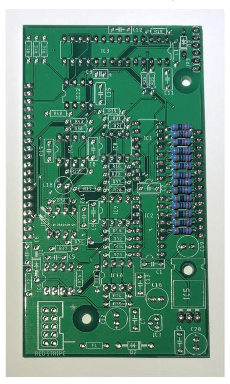
Install and solder the five 10K resistors R19, R21, R44, R45 and R46
