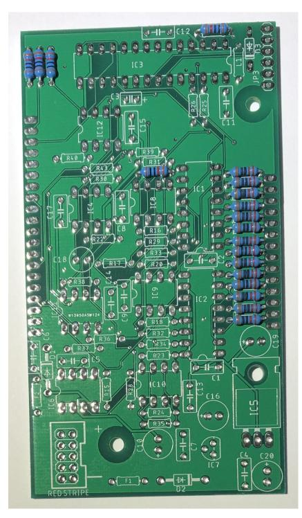
Install and solder the twelve 100K resistors R16, R17, R18, R20, R23, R24, R25, R26, R28, R30, R37 and R40  $\,$
