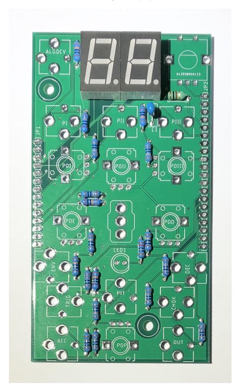
Cut the male header pin strip to size and solder in place, making sure it is at right angle to the PCB
