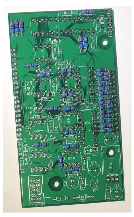
Install and solder the seven 150K resistors R29, R31, R32, R33, R34, R35 and R39
