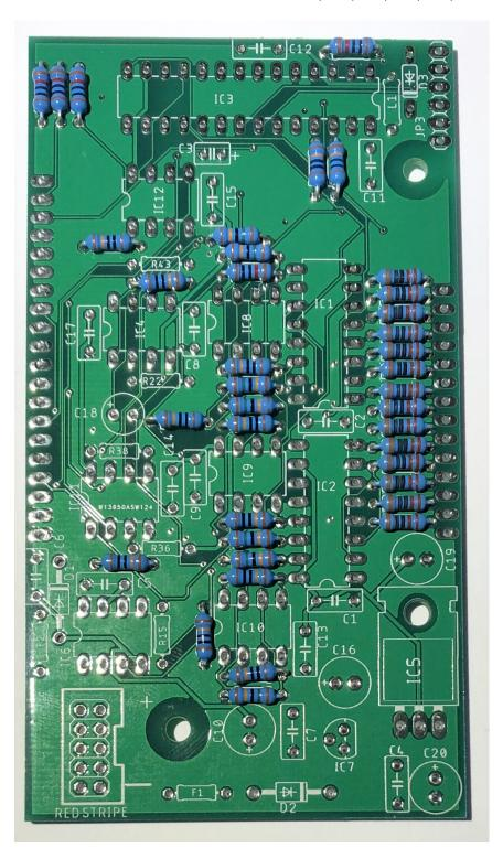
Install and solder the two 200K resistors R15 and R43
