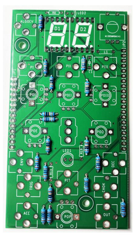
Install and solder the one 150K resistor R13
