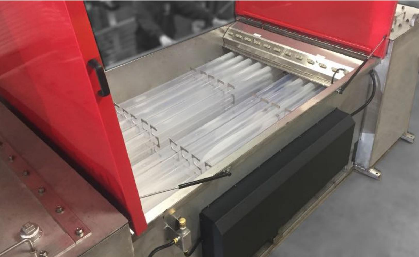
The “**NONCON 5000**” Series is a “flow through” fluoropolymer (aka FEP/Teflon™) style of ultraviolet (UV) water and wastewater disinfection systems.
