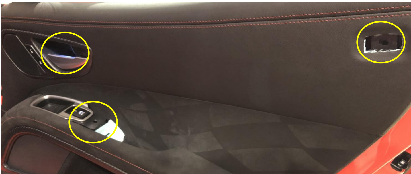
Gen 5 Door Panel Bolts on a 2017
