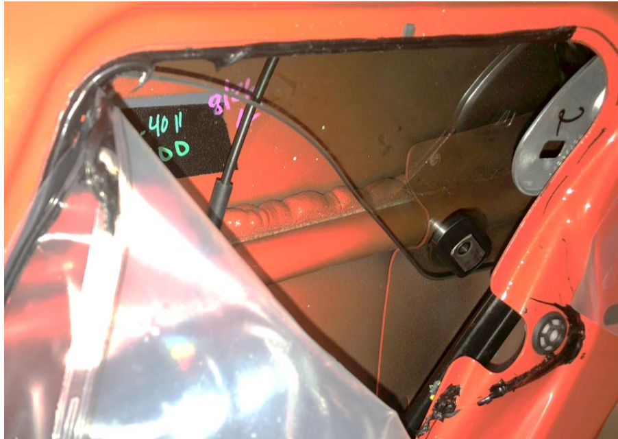
DSE Bosses Installed in Window Prior to Attachment to the Regulator
