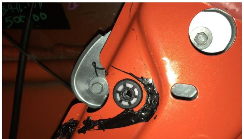
Peel back vapor barrier shown to allow access to window/regulator bolts
