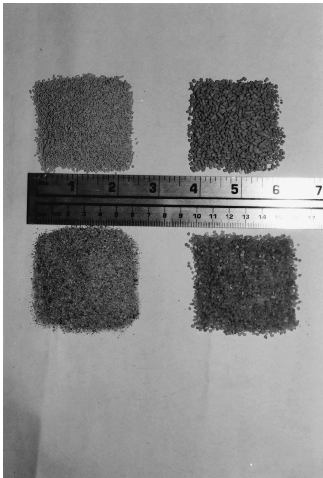
FIG. 1. Photograph of Constituent Materials Used in Sand–Diatomaceous Earth (DE) Mixtures: CG1 DE (Top Left); CG2 DE (Top Right); 20-60 Sand (Bottom Left); 10-20 Sand (Bottom Right)
