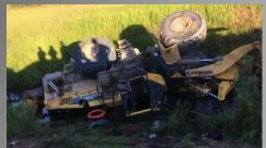
When his personal vehicle became stuck in a ditch, a miner decided to use a front-end loader to retrieve it. However, as he drove the loader toward the vehicle, he lost control, traveled through a berm and rolled over. The miner suffered serious injuries. The accident occurred on July 17, 2017.
