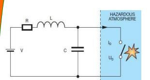
An intrinsically safe circuit is virtually incapable of generating arcs, sparks or thermal effects that are able to ignite an explosion of an explosive atmosphere, both during normal operation and during specific fault conditions
