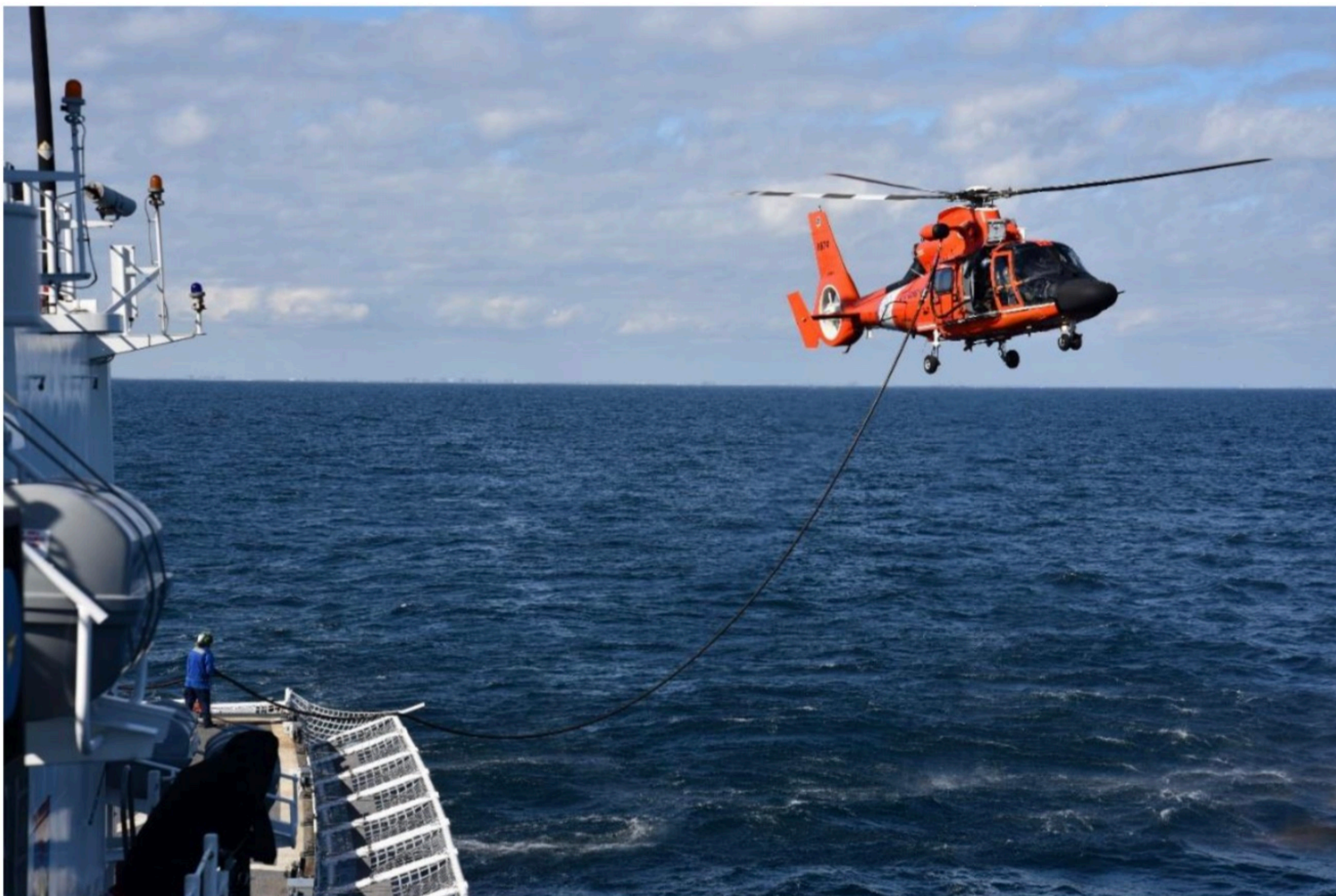
USCGC NORTHLAND (WMEC-904) Providing a Hot-In Flight (HIFR) to CG MH-65 Dolphin Helicopter.
