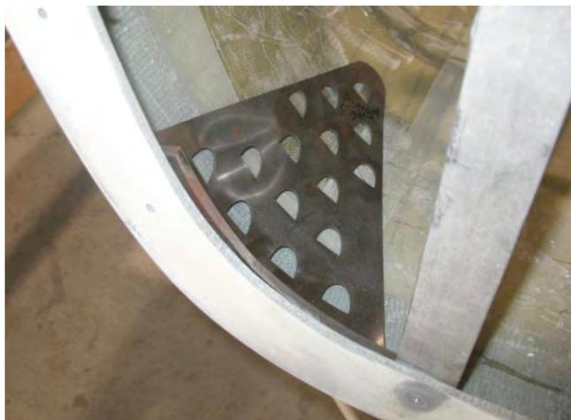
**Close up of an engine mount gusset for the larger HP engines. This one has not been bonded in yet, there is one at each fuselage engine mount attach point.**
