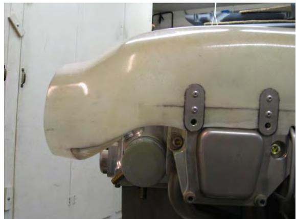
Maybe a little over kill, but this is my method of attaching the 'glass ducts. I prefer to back up the 'glass under the valve cover bolts with .032" aluminum.
