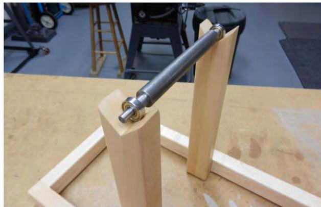
**Thanks Gary. Your homemade wheel balancer looks very similar to one that I use that was originally designed to balance go kart racing wheels. Buz**
