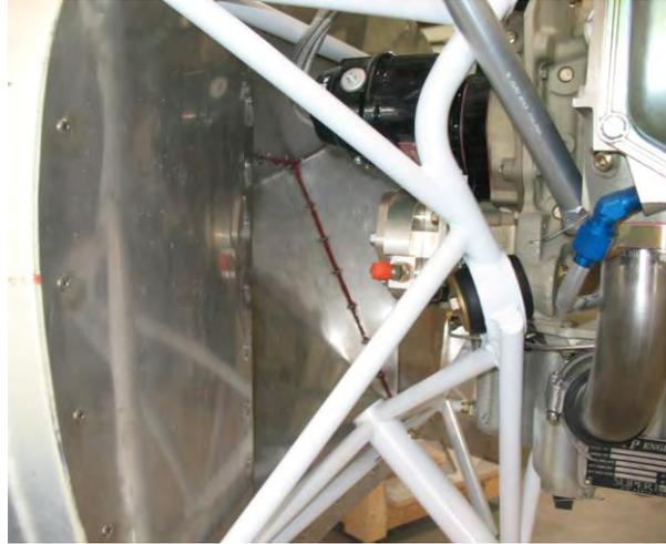
**These photos show a close up of a firewall recess area that was required to make space for O-320 engine accessories.**
