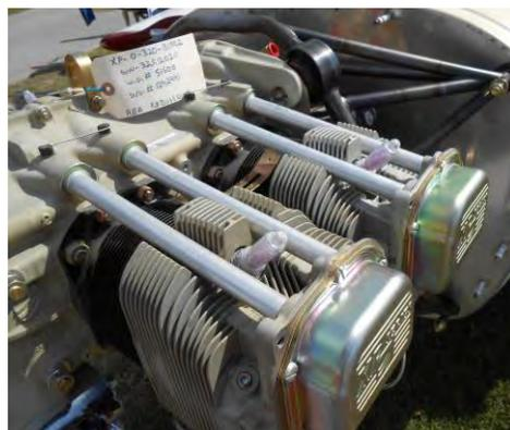
**Mark shows off the new 160 HP O-320 Lycoming. This thing is going to be fast. They may need a new airspeed indicator that is calibrated in mach numbers.**
