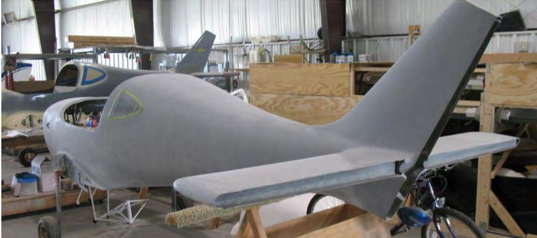
**This Lightning is being built by Doug and Ronda Guy; "Cornhuskers" from Nebraska. Their aircraft will be getting the UL390 160hp engine. The engine is here in a crate. It will be hung when the engine mount arrives here later this week.**
