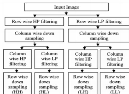
Fig.3 DWT decomposition
