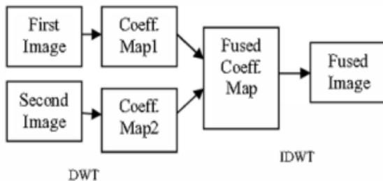
Fig.4 Image fusion process using DWT
