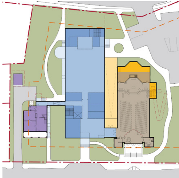
SCHEME 2: New Building on Existing Foundation
