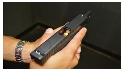
(Figure 8-2) Double Feed
