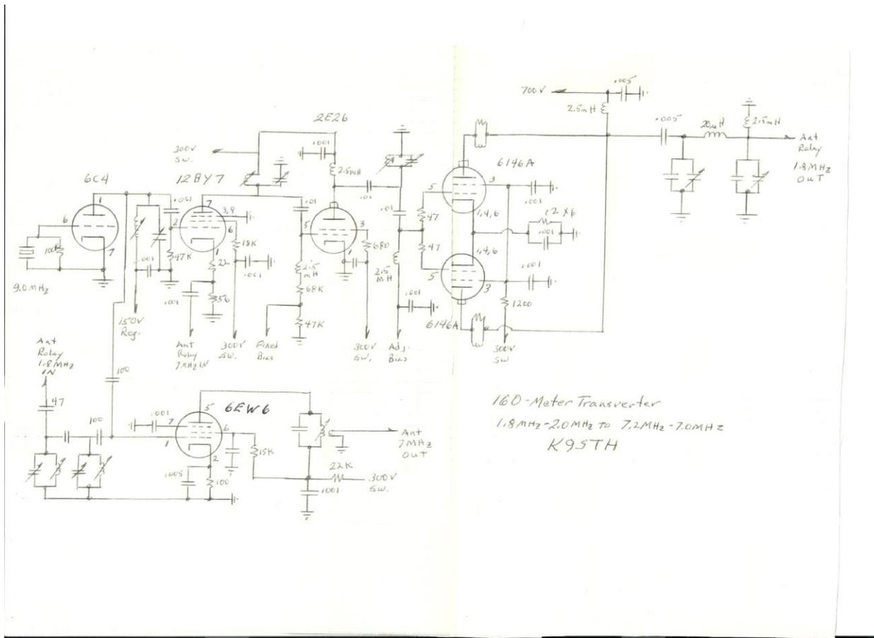
Schematic of 160-meter transverter. Only real difference between this and the final product is that the 6EW6 is now a 6DC6.
