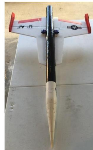
A major consideration in constructing this boost glider was to keep it light, to keep the wing loading as low as possible to maximize the glide slope. For adhesives, I used Foam Tac and foam-compatible CA. When attaching the wings and vertical stabilizers, I made fillets with medium CA and accelerator and was very happy with the results. The Center of Gravity (CG) for the liftoff/boost phase of this model should be at the intersection of the strakes and the main wing.
