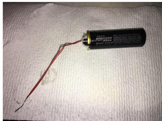
The E6 (E6-RCT, in the graphic below) motor is chosen for the Interceptor because it is a low thrust, long burn motor. As can be seen in the graphics, the E6 provides 40 N\*seconds (9 lb\*seconds) of total impulse with an average thrust of 6 N (1.2 lbf). The burn time of the motor is a little over 7 seconds. 21.5g (0.75 oz) of propellant will be consumed during the burn, meaning that the CG of the boost glider will move forward as the propellant is consumed.
