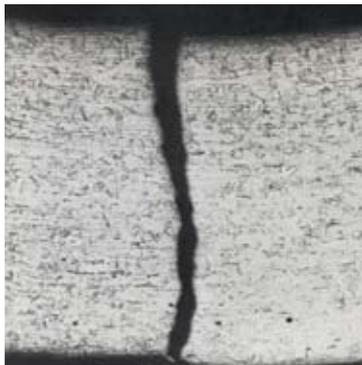
Figure 46. Fatigue crack.
