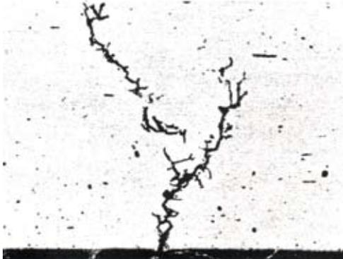
Figure 45. Photomicrograph of intergranular stress corrosion cracking.
