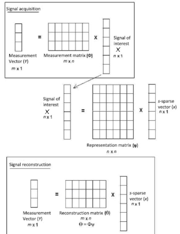
Fig 1. Computational Model of the Compressed Sensing
