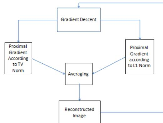
Fig 2: The reconstructed image is obtained from missing solution of the sub problem in a repetition passion.
