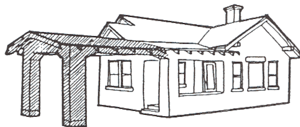
Addition of porte cochere or carport using similar roof form, scale and architectural features.
