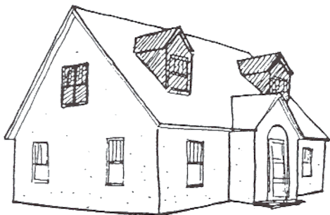
Conversion of attic space to living area with the addition of appropriately scaled dormers.
