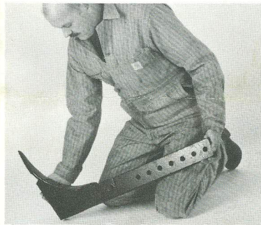
The straight, lighter chisel is designed for moist or loamy soil conditions, or for Spring soil preparation. Chisels are adjustable from 3" to 9" below the Rotor blades.
