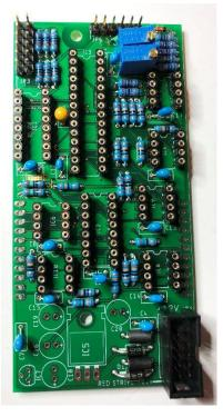
Install the two voltage regulators IC5 and IC7
