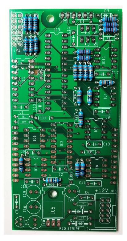
Install and solder the six 150K resistors R29, R31, R32, R33, R34 and R35
