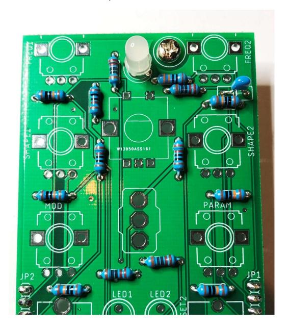
Seat the encoder, pots and switch followed by the jacks and LED's. DO NOT SOLDER ANYTHING ... yet!! NOTE: there is a nut on the encoder to act as a spacer between the panel. Put the nut on before seating as its very fiddley doing it once its on the PCB with all the other parts.
