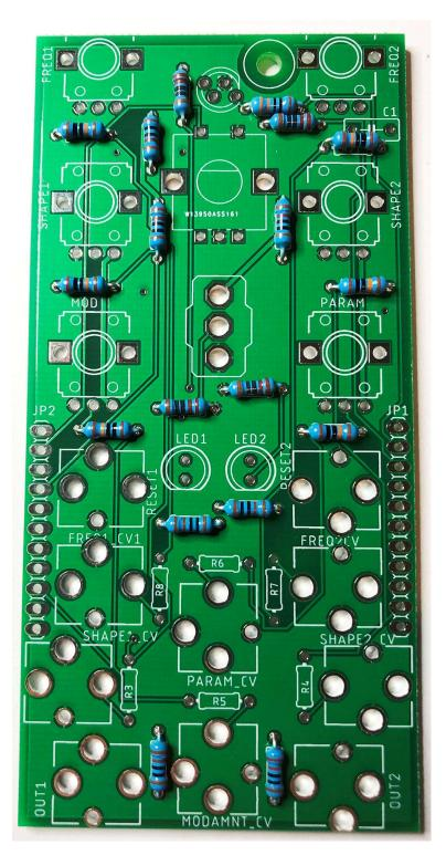
Install and solder the six 200K resistors R3, R4, R5, R6, R7 and R8
