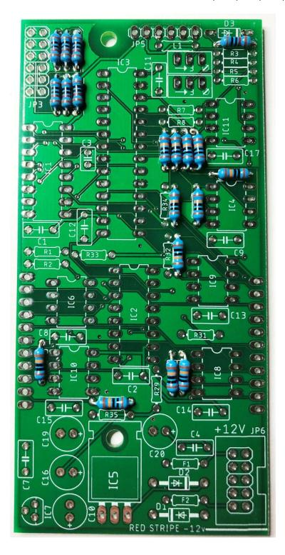
Install and solder the four 22K resistors R3, R4, R7 and R8
