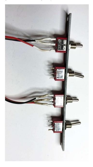
Repeat the same process for the 2-wire pieces, this time connecting them to the center and the bottom lug of the ON-ON switches (LFO/Ramp selector). Be sure to use the same colours on the same lugs to make connection easier.
