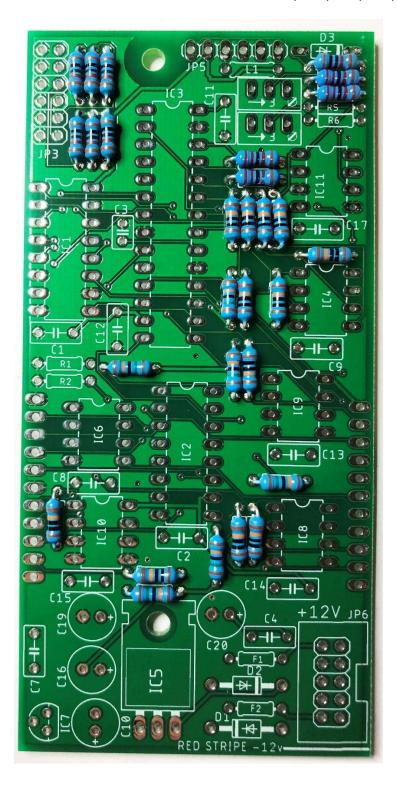
Install and solder the two 200K resistors R5 and R6
