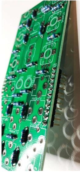
Install and solder the RGB LED. Make sure that the flat side of the LED aligns with the silk screen. The longer pin is the cathode and is marked on the silk screen with a square. Make sure the LED is as close to the board as possible – this requires applying a little bit of GENTLE force, but not so much that you bend the LED. If you do bend the LED, straighten it and make sure no pins are touching.
