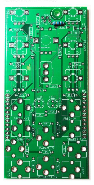
Install and solder the four 220R resistors – R12, R13, R14 and R16
