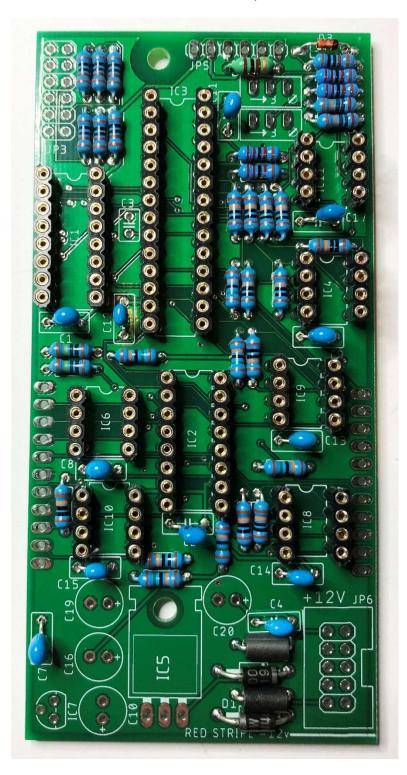
Install and solder the two 100K 25-turn trimmers. Cut the remaining male pin header into three 6 pin pieces and install and solder them into JP3 and JP5
