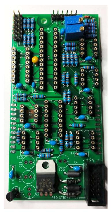
Install the four 100uf electrolytic capacitors C10, C16, C19 and C10 paying attention to the polarity (long pin is positive, stripe on the capacitor is negative).
