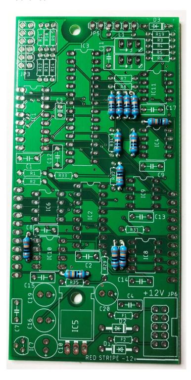
Install and solder the seven 10K resistors R9, R10, R11, R12, R13, R14 and R19
