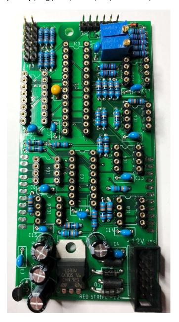
Cut the female header strip into two 11pin pieces and install and solder them.
