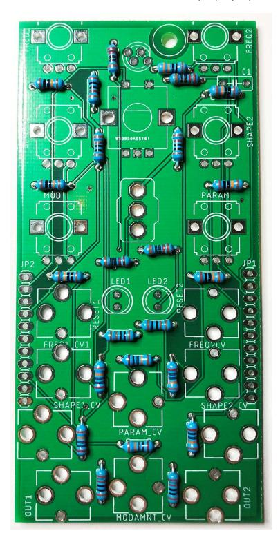
Cut the header pin strips to size (11 pins in length) using side cutters or pliers. Install and solder making sure they are at right angles to the board.
