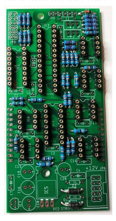
Install and solder the two axial ferrite beards F1, F2 and the inductor L1
