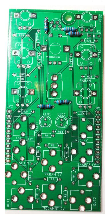
Install and solder the six 100K resistors R20, R21, R22, R23, R24 and R25
