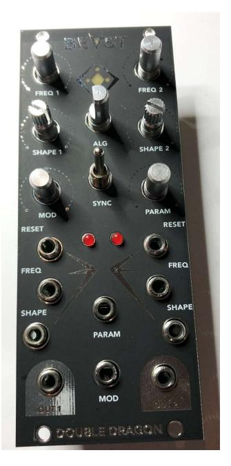
Place the nut on the switch, washer and nut on the encoder and two knurled nuts on two of the jacks. Finger tighten the encoder nut and firmly tighten the switch and jack nuts. This should be enough to hold things together so you can flip it over and solder everything in place. For me this was very firm and things were not falling apart. Its possible that you may have to install more knurled jack nuts or washers+nuts on the pots to keep things together.
