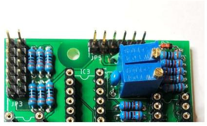
Install and solder the 10uf tantalum capacitor paying attention to the orientation of the positive pin as per the photos below
