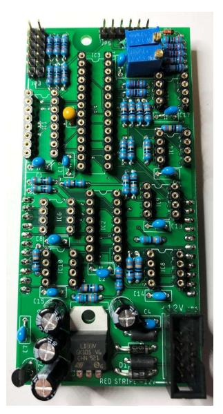
Install the TL072 IC into IC11
