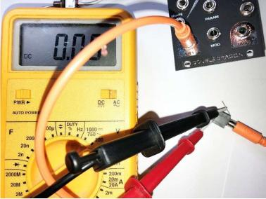
The trimmer closest to the top of the module adjusts the zero offset for OUT 1 and the trimmer closest to the bottom of the module adjusts the zero offset for OUT2.
