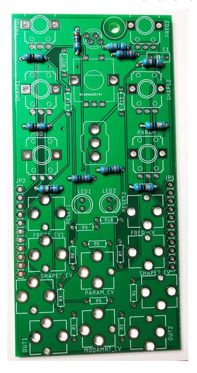
Install and solder the three 10K resistors R17, R18 and R19
