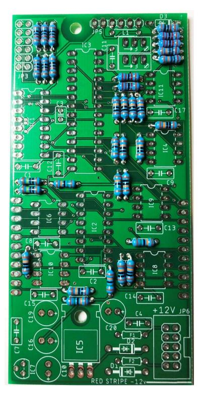
Install and solder the two 1N4004 diodes D1, D2 and the 1N4148 diode D3 – paying attention to the band on the diode and the silkscreen on the board.
