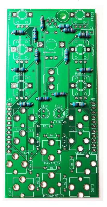
Install and solder the four 1K resistors R1, R2, R9 and R10
