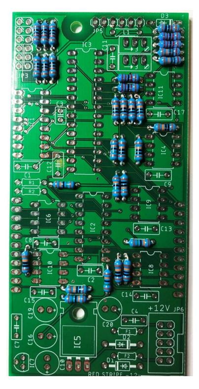
Install and solder the two 1M resistors R1 and R2
