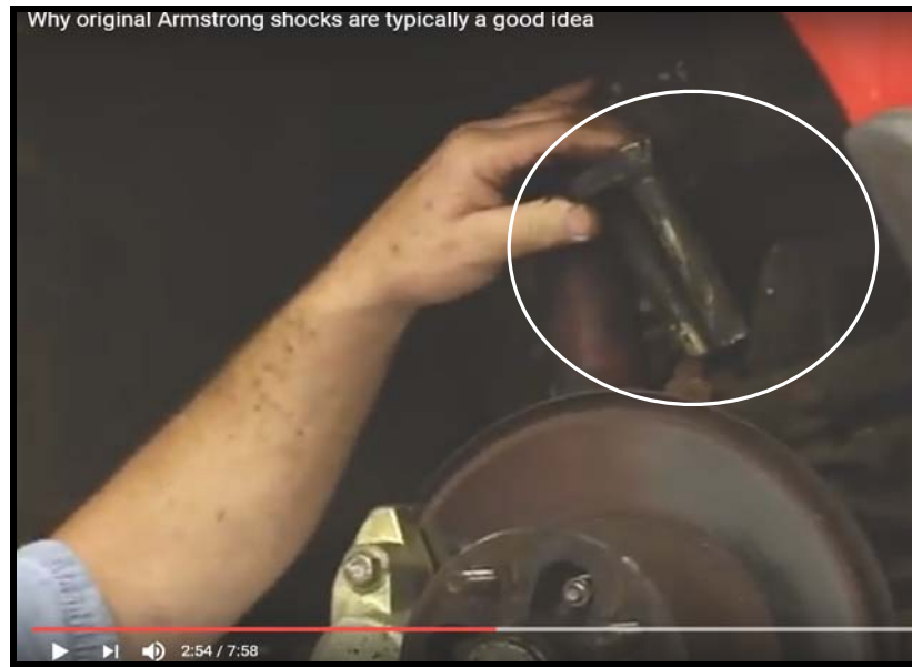
Figure 36 - Damaged Support Bracket
