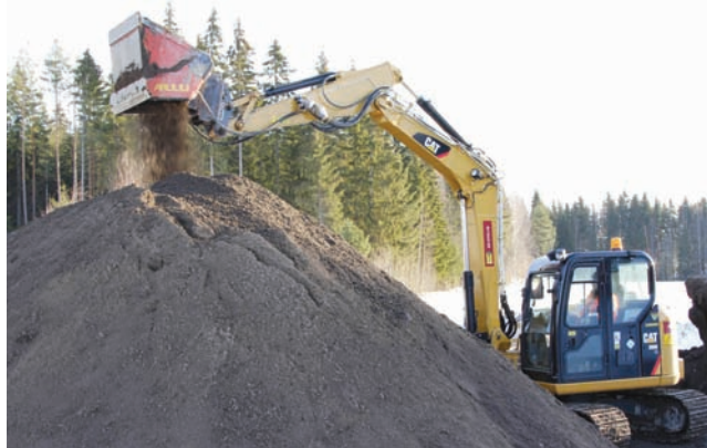
The DL 2-12 bucket is recommended for compact excavators weighing 15,400-26,000-pounds and for small wheel loaders weighing 6,600-17,600-pounds.
