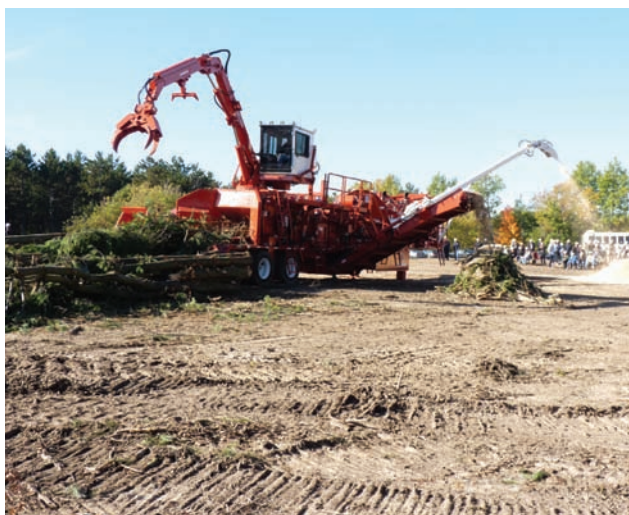
The 2755 Flail Chiparvestor was being demonstrated with the railcar loading chute (the white discharge chute on the right).
