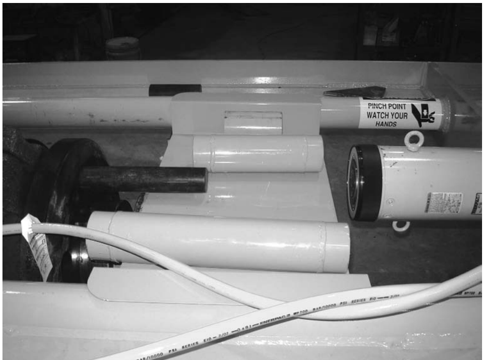
Side view of 100 ton press. Note the tray that allows easy rolling in of various length spacers that match the 100 ton cylinder stroke length to push the rod out.
