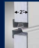
Tongue-and-groove construction is used in the manufacturing of all 2500 series doors. The door shown includes optional polystyrene insulation panel. (exterior cross section view)
