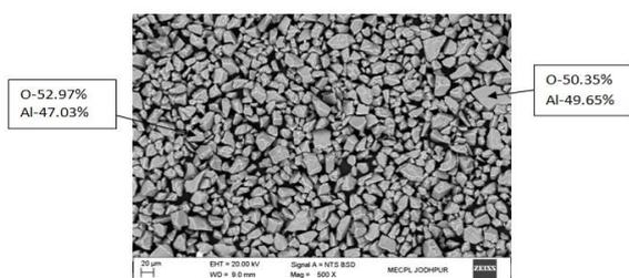
Fig.1 SEM/EDAX analysis of Al<sub>2</sub>O<sub>3</sub> coating powder showing elemental composition (% wt)
