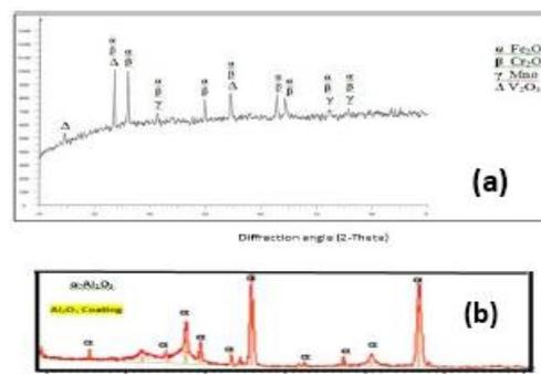
**Fig 6** X-ray diffraction patterns for (a) uncoated ; (b) coated T-91 steel subjected to oxidation in air for 50 cycles at  $700^\circ\text{C}$
