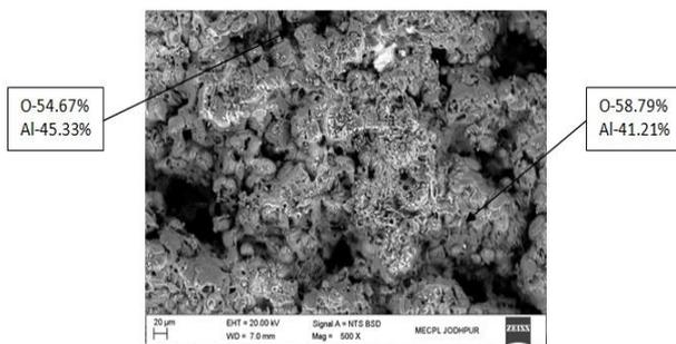
Fig. 3 SEM micrograph and EDAX analysis of Al<sub>2</sub>O<sub>3</sub> coating on T-91 showing elemental composition (% wt) at selected points
