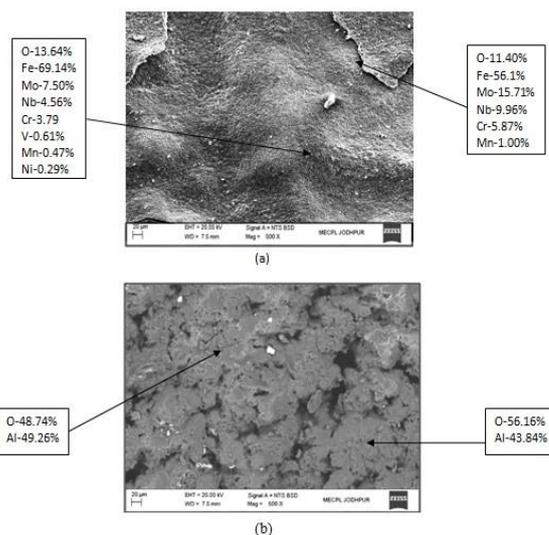
**Fig.7** SEM micrographs and EDAX analysis of uncoated and coated T-91 subjected to oxidation in air for 50 cycles at  $700^\circ\text{C}$  (a) Uncoated T 91 (b)  $\text{Al}_2\text{O}_3$
