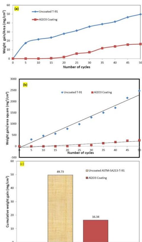
**Fig 5** (a)Weight gain/Area vs number of cycles plot (b)(Weight gain/Area)<sup>2</sup> vs number of cycles plot (c) Cumulative weight gain bar chart for uncoated and Al<sub>2</sub>O<sub>3</sub> coating on T-91 substrate steel subjected to high temperature oxidation in air for 50 cycles at 700°C
