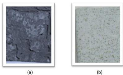
**Fig.4** Macrographs of uncoated and coated substrate T-91 steel subjected to oxidation in air for 50 cycles at 700° C (a) Uncoated T-91 (b) Al<sub>2</sub>O<sub>3</sub>
