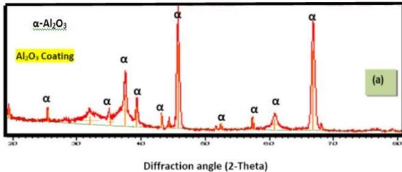
Fig.2 X-ray diffraction patterns for Al<sub>2</sub>O<sub>3</sub> coating on T-91 steel
