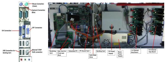
Figure 13 – Monitor, Keyboard and Mouse Direct Connection
