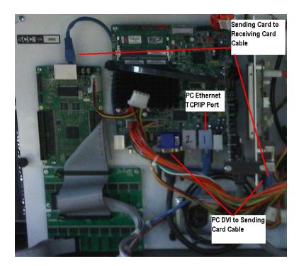
3. Check ribbon cable connection from receiving card to hub cards (front and back).
