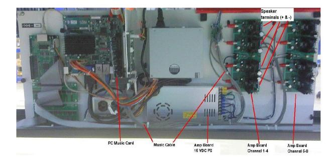
5. VNC into boards PC to check OPCDVI program for volume settings, and that tune is active for suspect music channel (Unit 2 =Chan 1).
