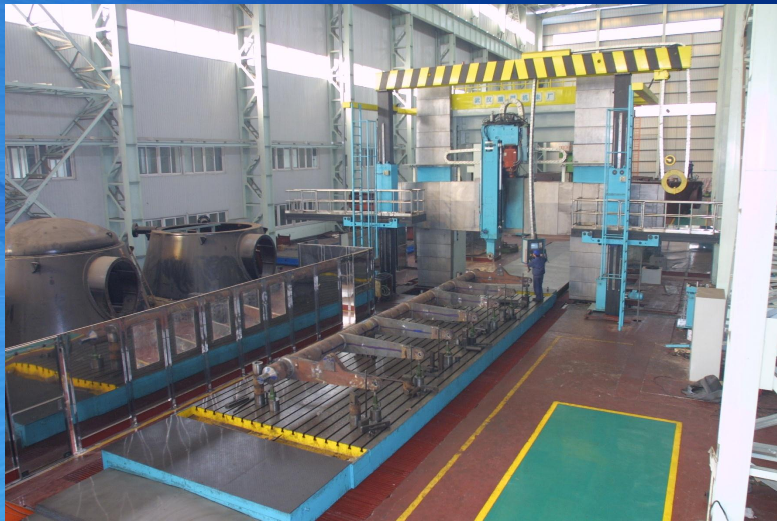
数控龙门镗铣床 XK2140×120 CNC planer Type Boring and Milling Machine
