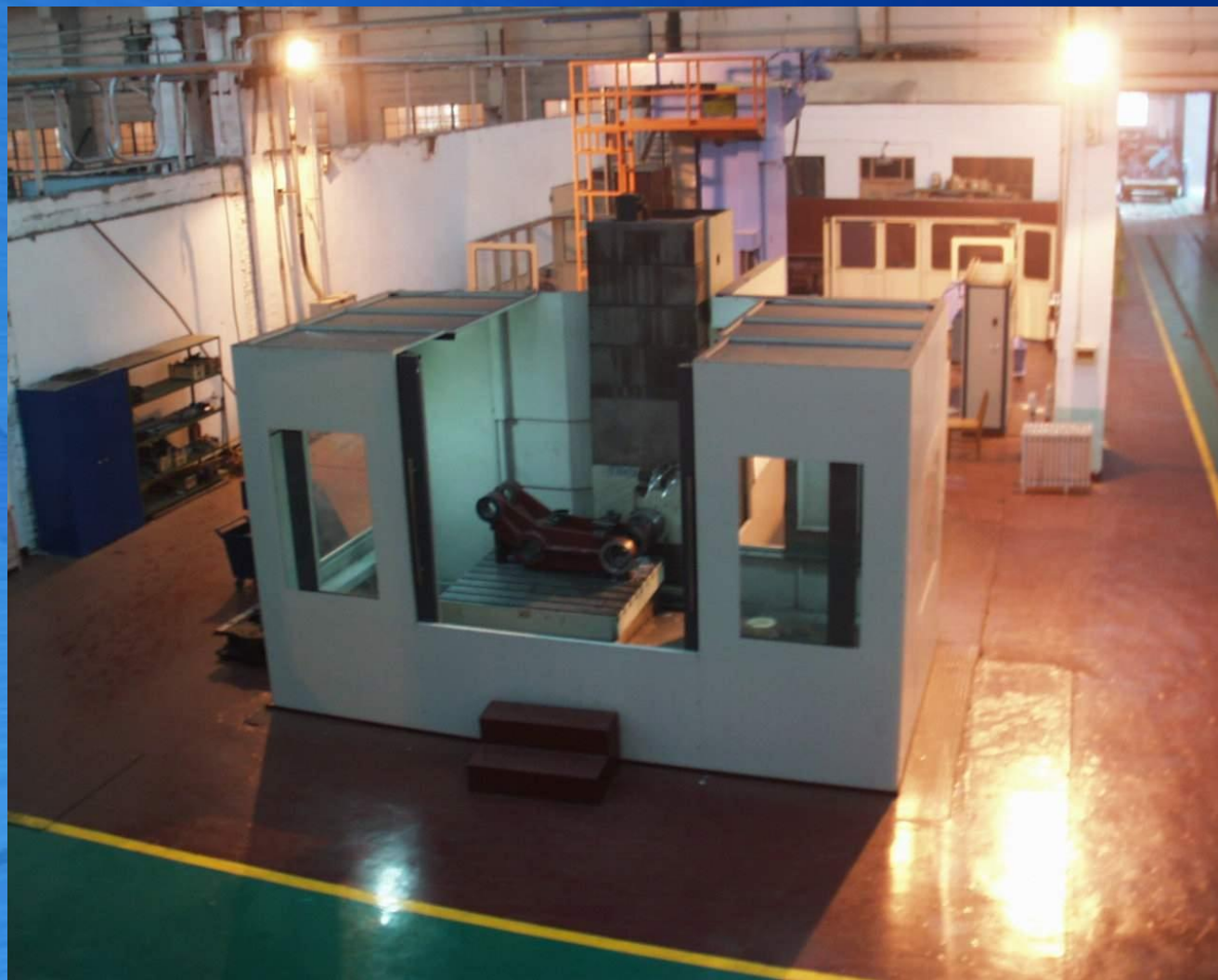
数控卧式铣镗加工中心 TH65140×160B/3D CNC Horizontal Machining Center TH65140×160B/3D
