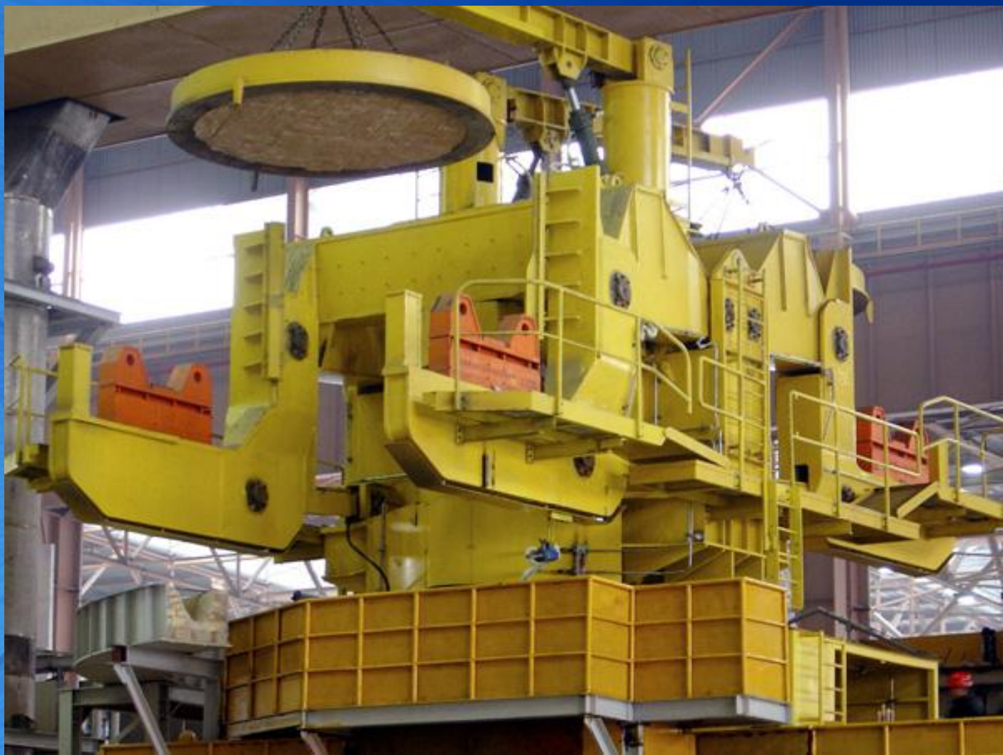
90吨钢包回转台 90t Rotary table of ladle
