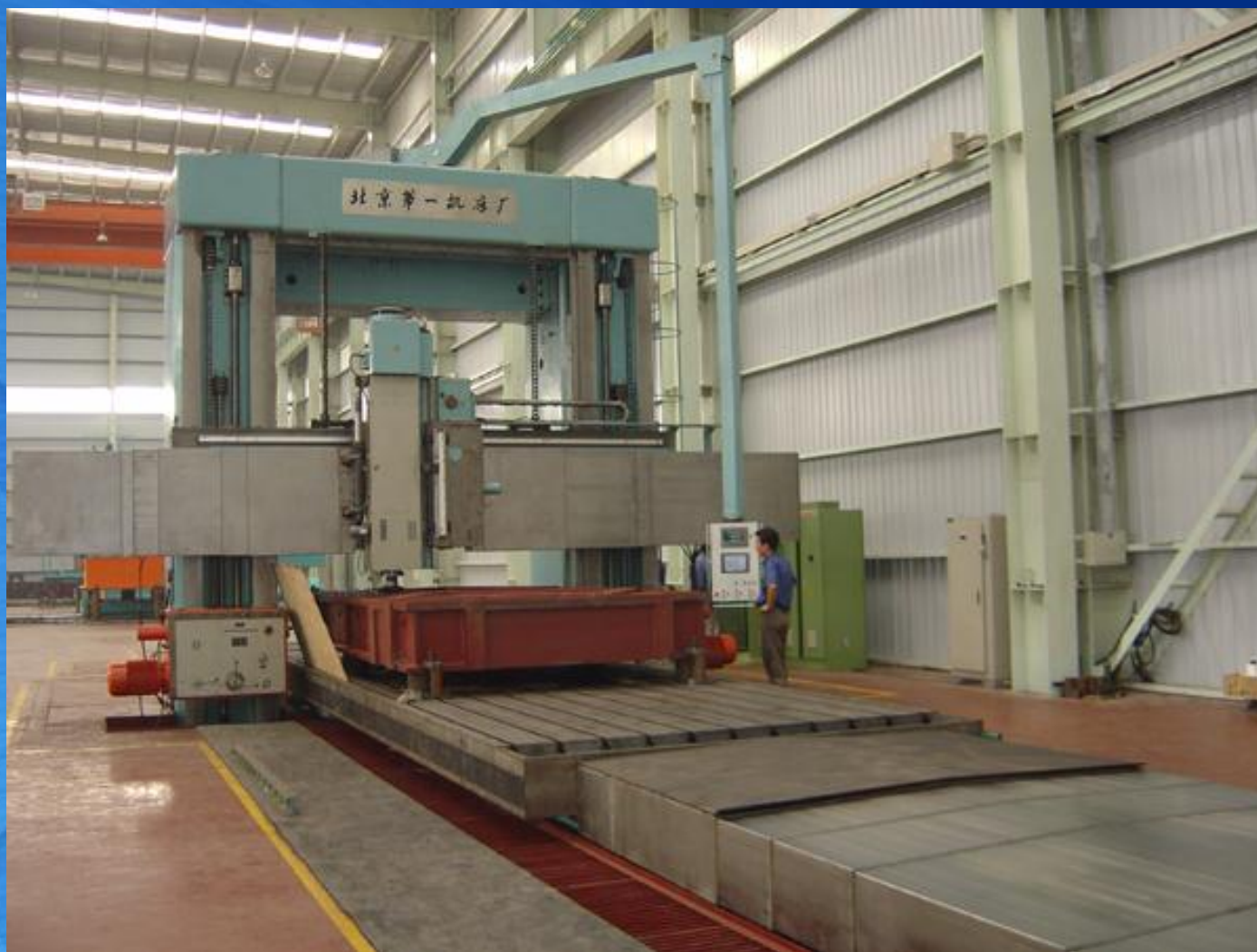
数控龙门镗铣床 型号: XA2130(2.6)×100A/5 CNC planer Type Boring and Milling Machine
