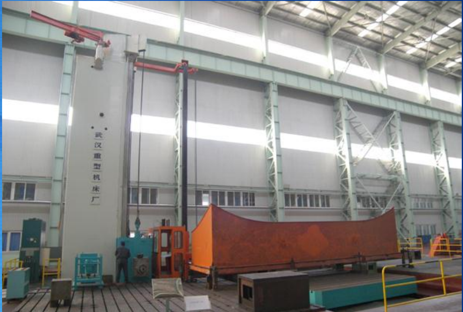
FB260/180 数控落地铣镗床 CNC Boring and Milling Machine
