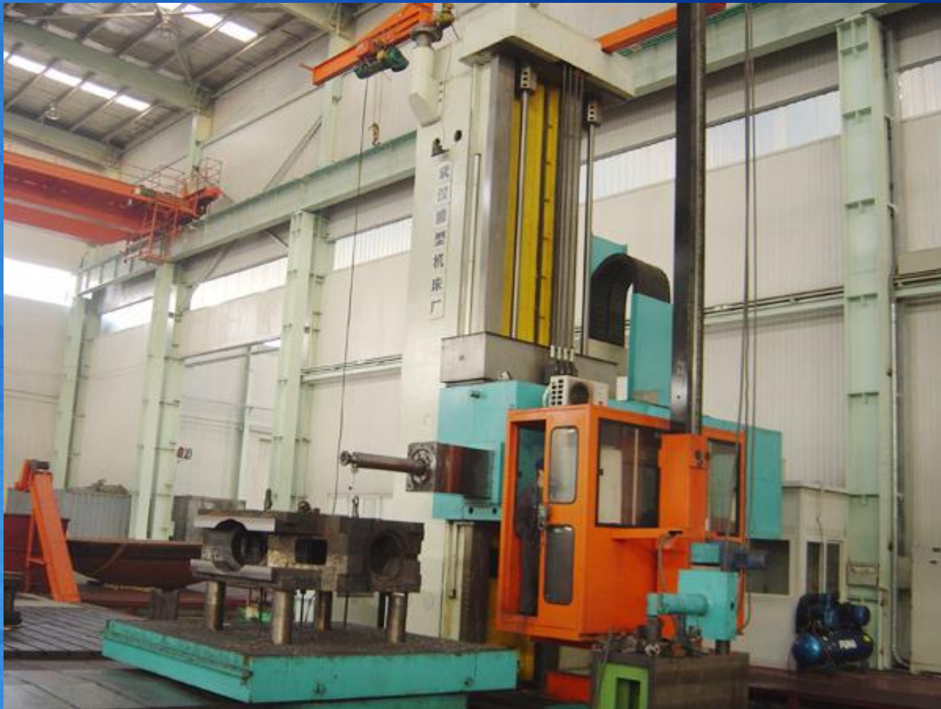
数控镗床Tk6916B/150X50 CNC Console Boring Machine Tk6916B/150X50
