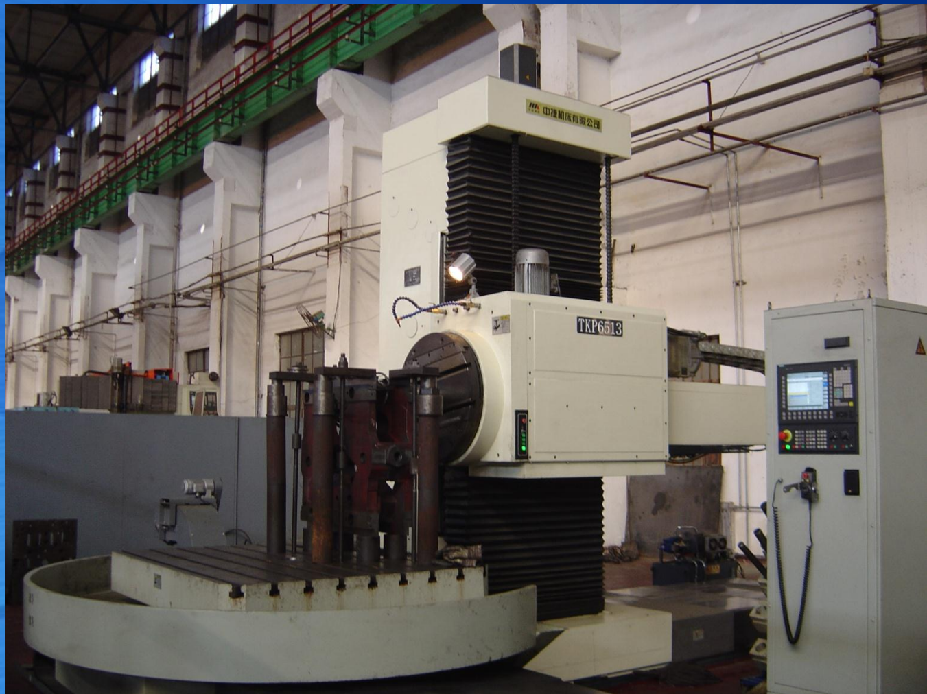
TKP6513 数控刨台卧式镗铣床 TKP6513 CNC Horizontal Boring and Milling Machine
