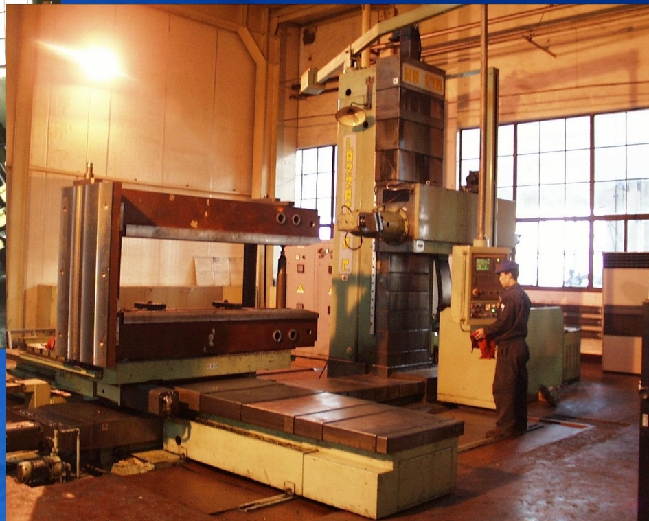
意大利HB130数控镗铣床 Italian HB 130 CNC Boring and Milling Machine
