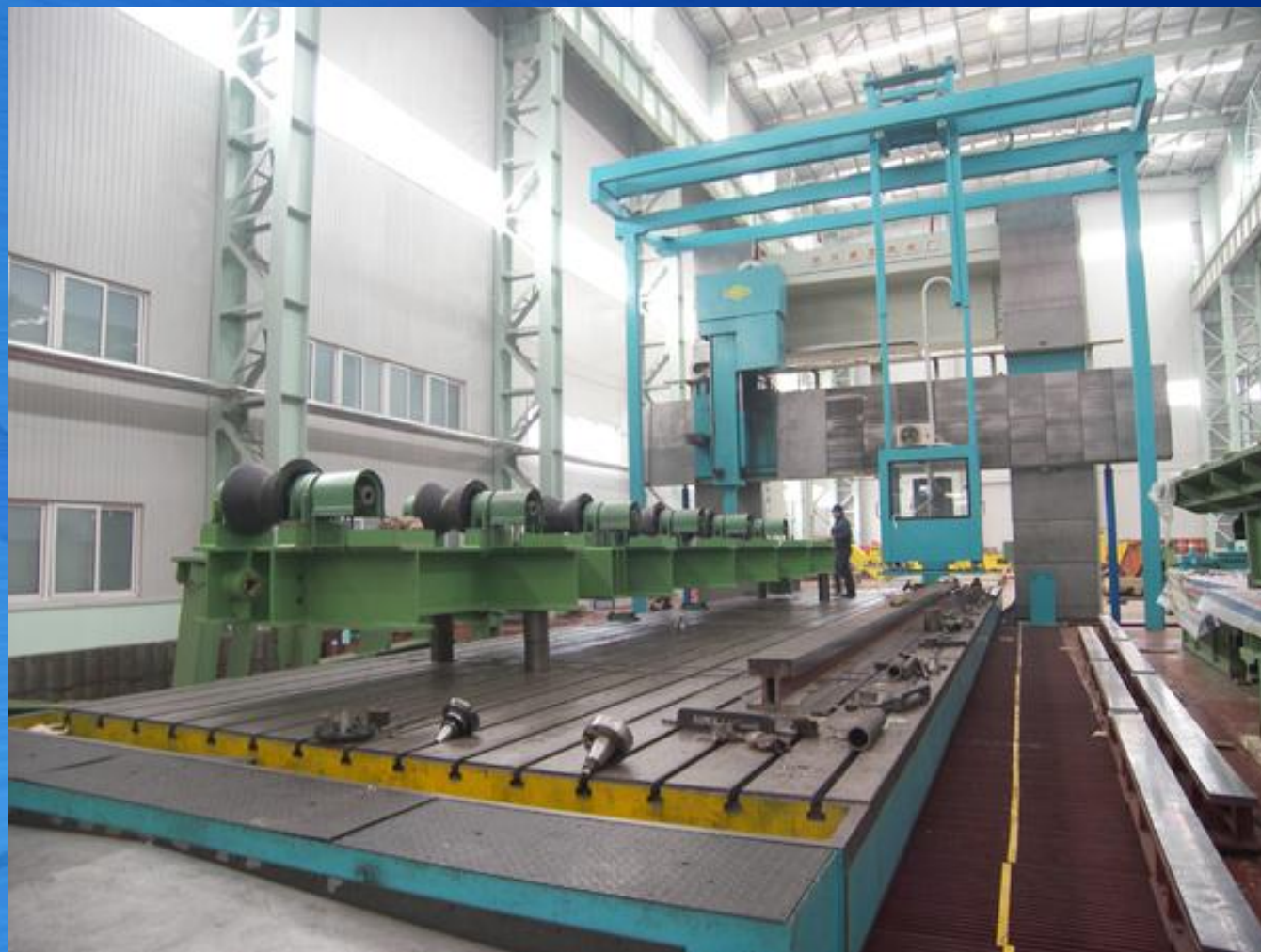
数控龙门镗铣床 XK2150×180 CNC planer Type Boring and Milling Machine XK2150×180
