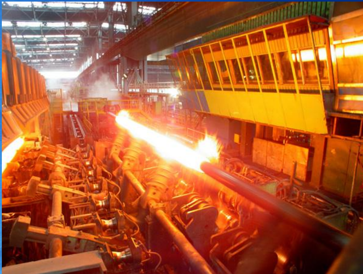
轧管生产线 Production Line of Rolling tubing
