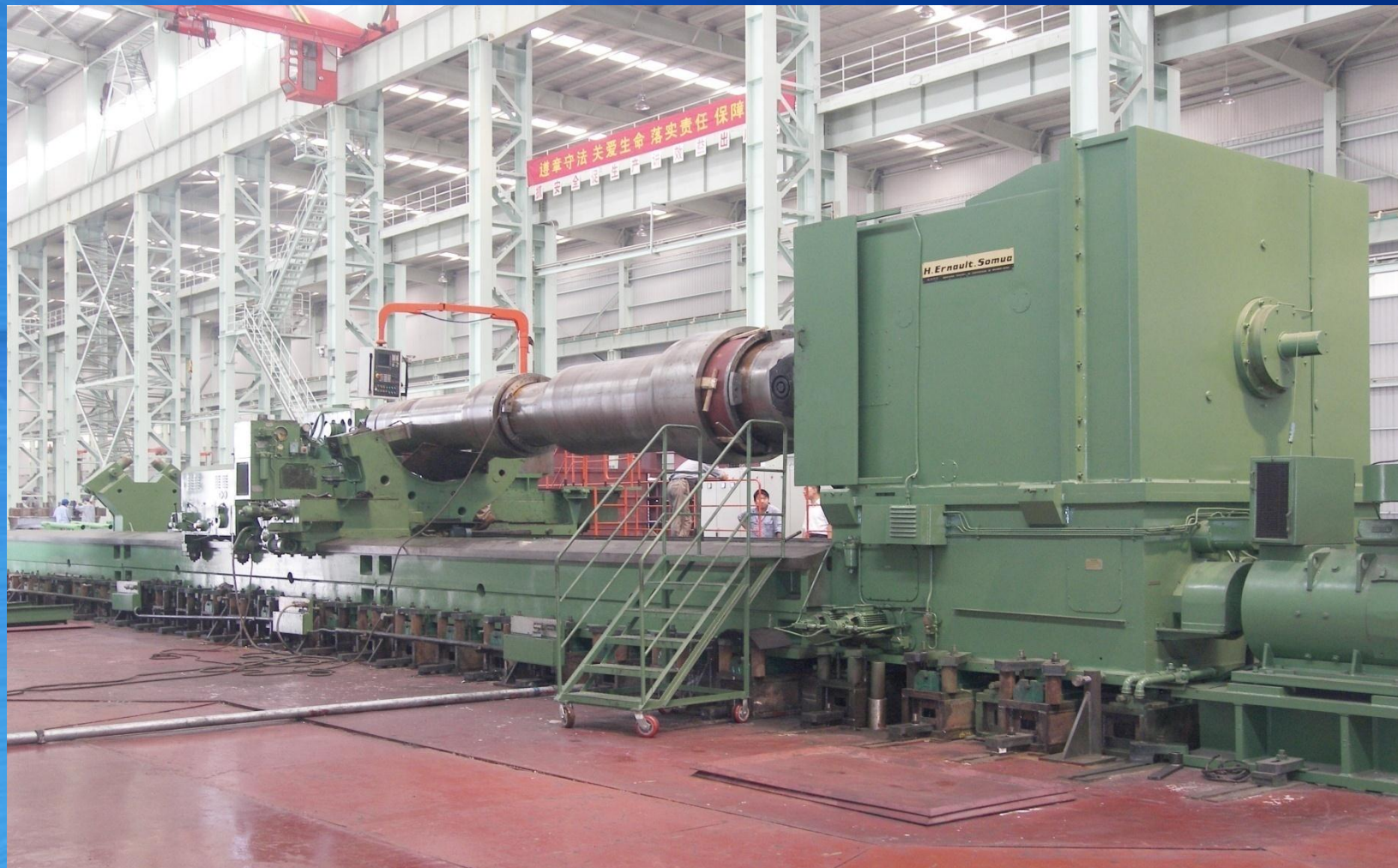
2800x18000mm 数控卧式车床 2800x18000mm CNC Horizontal Lathe
