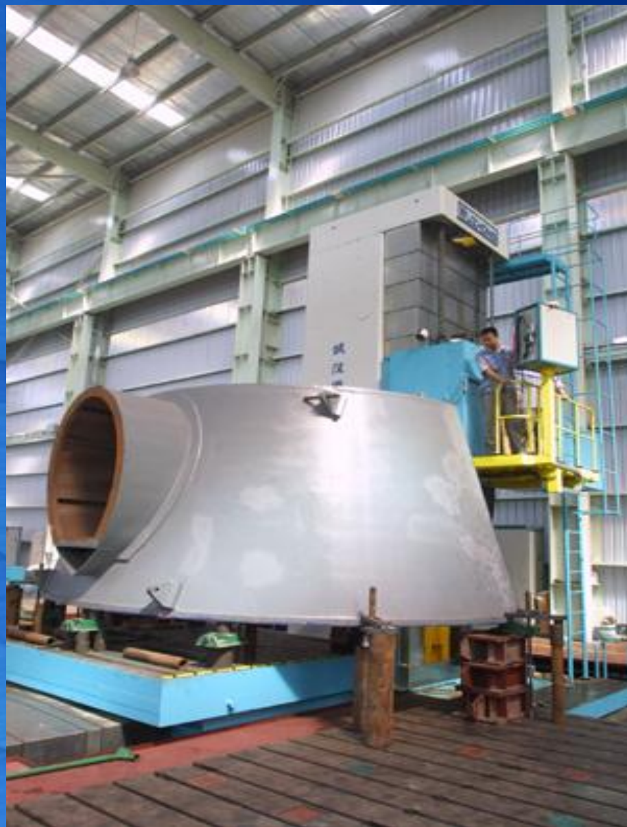
数控落地镗床 TK6916A CNC Console Boring Machine TK6916A
