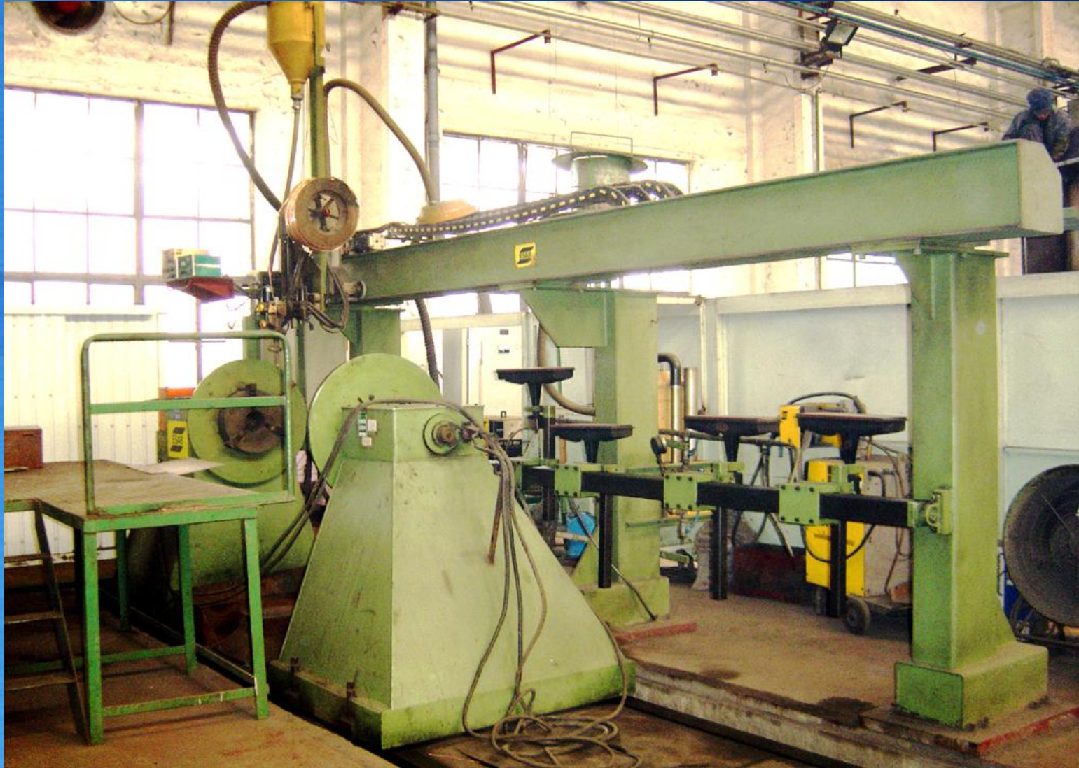
ESAB 自动埋弧焊接装置 ESAB Automatic Submerged Arc Welder
