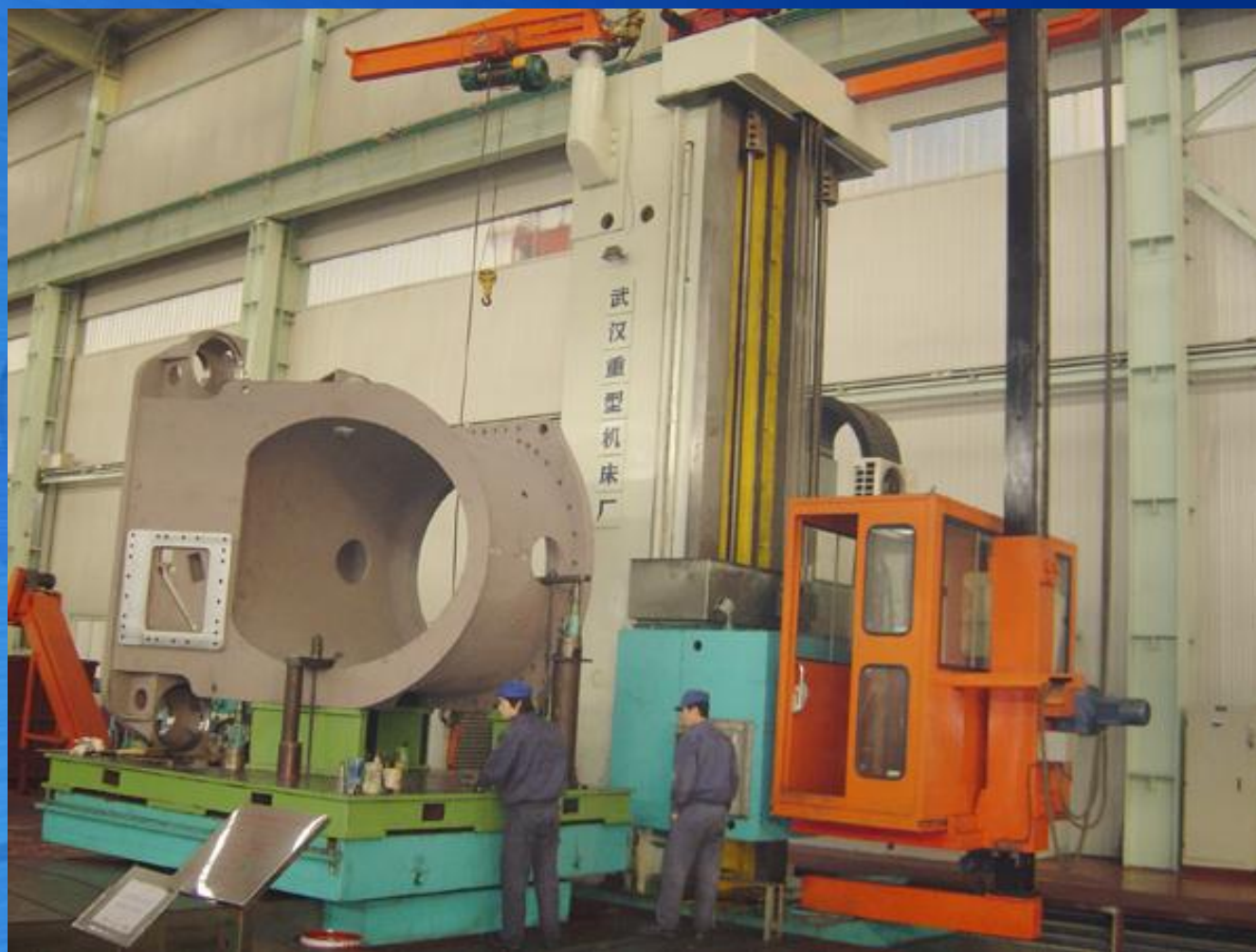
数控镗床Tk6916B/100X40 CNC Console Boring Machine Tk6916B/100X40
