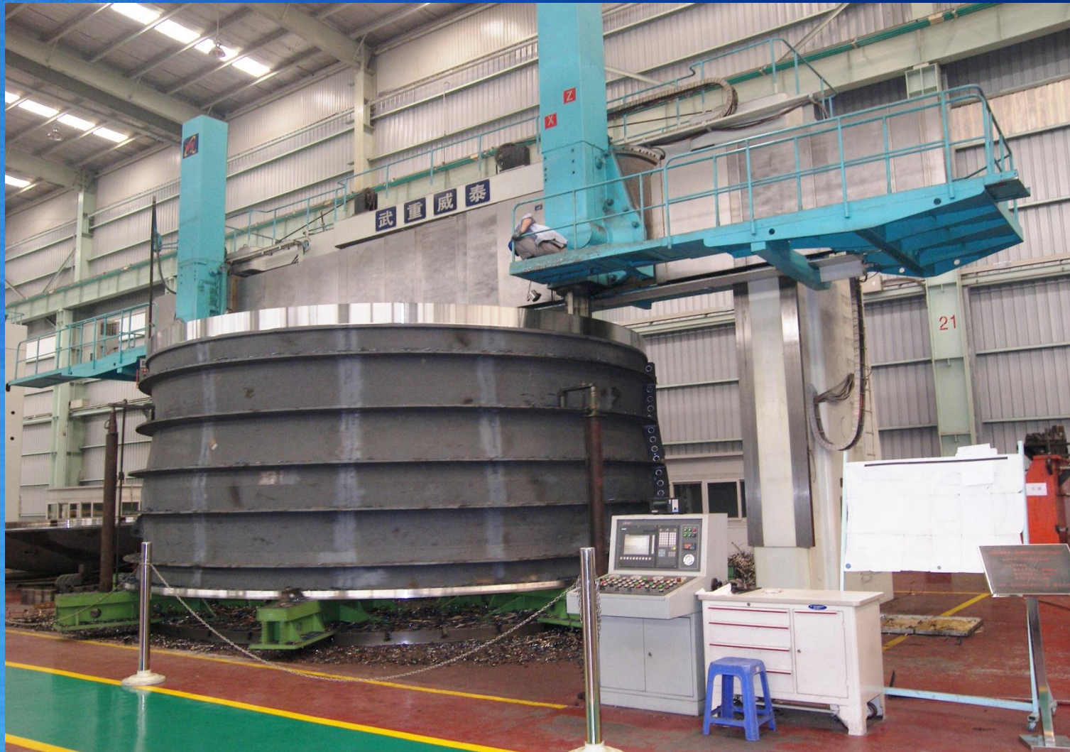
转轮室（铜湾水电站项目） Tongwan Hydro-power Runner Housing
