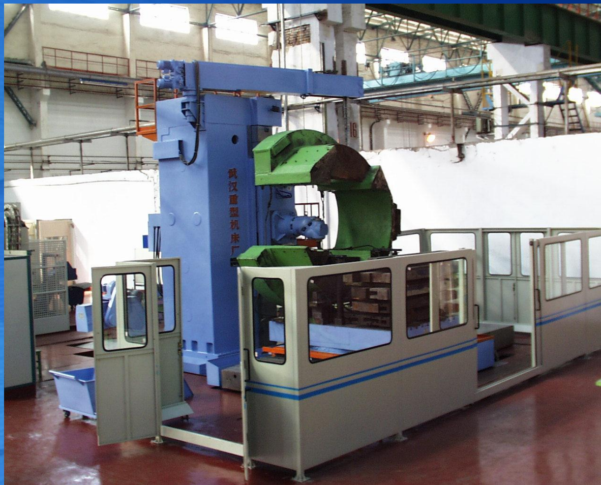
数控卧式刨台镗铣床 CNC Horizontal Boring and Milling Machine
