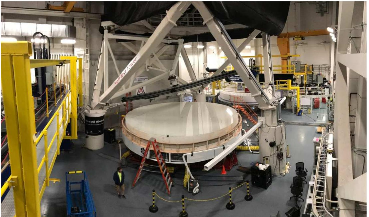
*Underneath the Stadium. Mirror 1, in foreground, undergoing final testing. Mirror 4 in background. Note the worker at bottom left for a sense of scale.*
