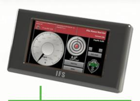
7" Windows OS LCD touchcreen in a rugged ABS casing. Designed to IP67 ingress protection.
