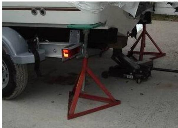
A powerboat on the trailer with boat stands positioned on back of hull right underneath the transom.
