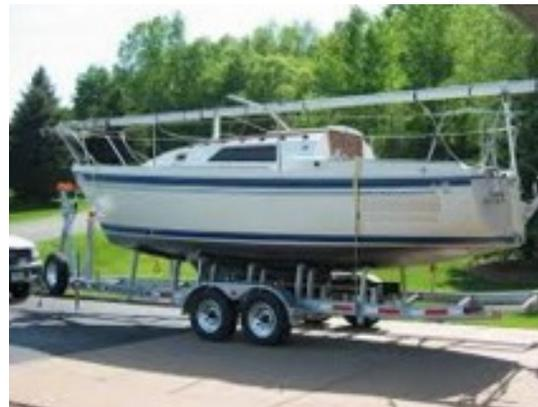
A sailboat clearly showing trailer bunks not running to complete rear or front of the whole exposing free space for lifting straps to be placed under the hull.
