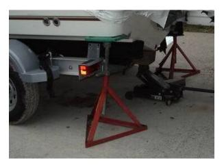
A powerboat on the trailer with boat stands positioned on back of hull right underneath the transom.
