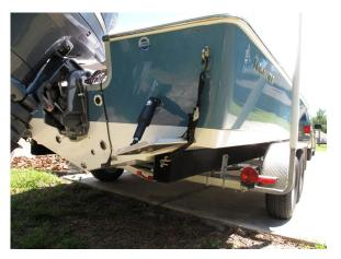
A powerboat showing the aft of the boat on a trailer with locations on the back hull that are not obstructed by the trailer allowing for boat stands to be placed directly on the bottom of the boat's transom.
