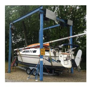
A sailboat positioned in a stationary hoist and shows the exposed rear hull that allows straps to be placed under.
