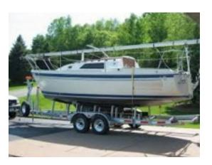
A sailboat clearly showing trailer bunks not running to complete rear or front of the whole exposing free space for lifting straps to be placed under the hull.
