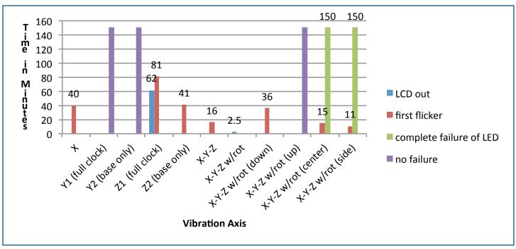
FIGURE 15 - TIME TO FAILURE VS. AXIS
