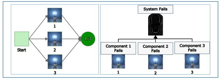
FIGURE 2 - SYSTEM RBD AND FT FOR A 1-OUT-OF-3 PARALLEL SYSTEM
