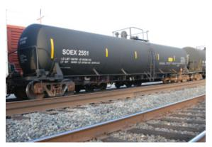
Oil Tank cars on 2nd St. in Davis on Jan. 9, 2014. #1286 means petroleum distillates classified at level 3, highly flammable liquid, same category as crude oil.
