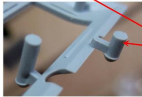
Ejection Pin Marks (some recessed, some raised, some off the part)
