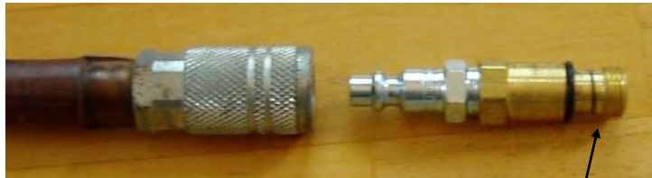
Spark plug hole adapter w/ 12 MM threads
