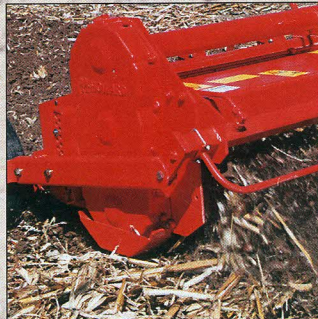
Rotavator is the most effective system for crumbling and residues incorporation.
