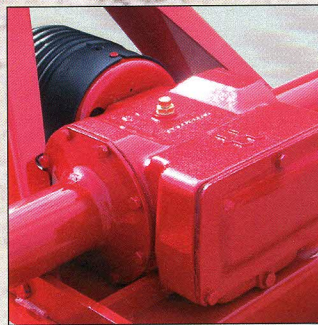
Standard Selectatilt gearbox. The speed is adjusted to the desired finish.
