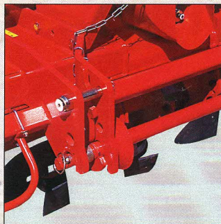
Linkage cat. 3 and 2 with quick coupling.
