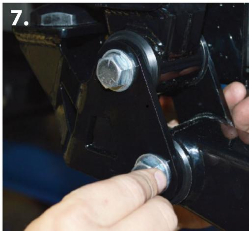
9. Assemble shackles and frame mount brackets with provided bump stops, bushings, and sleeves.
