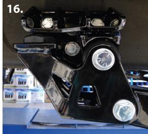
20. Now fully assemble shackle and traction bar back onto the frame mount. (pic 16) 21. Be sure to check the entire vehicle to make sure nothing is rubbing. Check all tires, brake lines, hoses, sensors, wires, etc, for clearance. Tighten ALL hardware on traction bars at this time.
