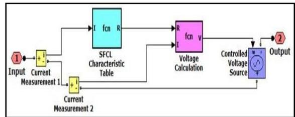
Fig 6a- DC-SFCL model in Simulink
