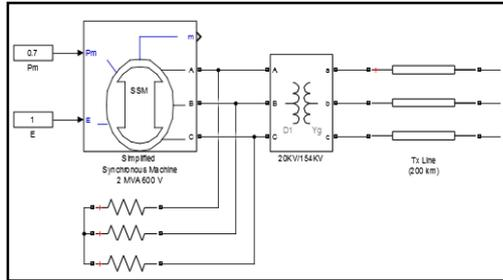
Fig 7a- 3-phase Synchronous machine
