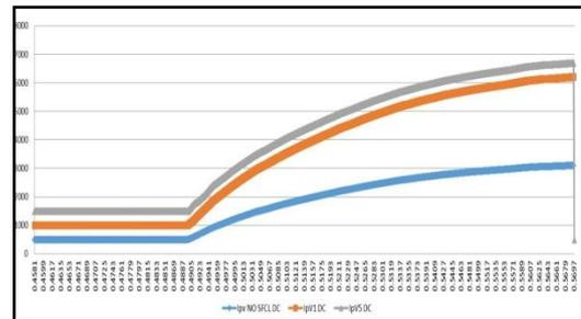
Fig. 11 -Comparison of the Photovoltaic Farm fault currents for different SFCL locations in case of fault in DC microgrid.
