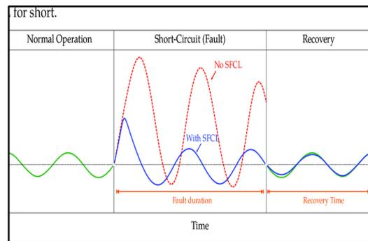
Fig.1. Characteristics of Fault Current Limiters into three operating modes
