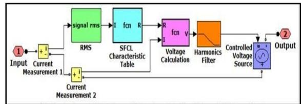
Fig 6b- AC-SFCL model in Simulink
