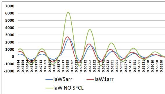
Fig. 10a-Comparison of the wind farm fault currents for different SFCL locations in case of fault in AC microgrid
