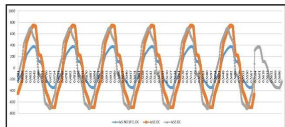
Fig.12-Comparison of the substation transformer fault currents for different SFCL locations in case of fault in DC microgrid.
