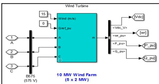
Fig 8a- Wind power generator system
