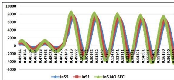
Fig. 10b-Comparison of the substation transformer fault currents for different SFCL locations in case of fault in AC microgrid
