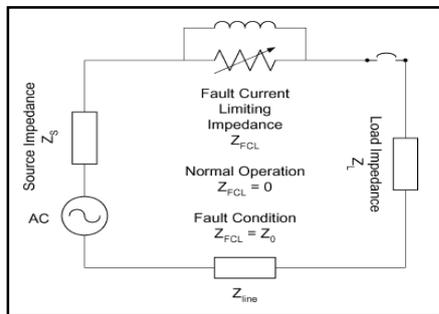
Fig.4. Equivalent circuit of SFCL in a power system
