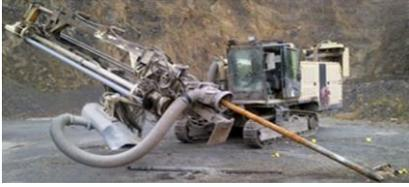
In fact, at least seven workers died in metal and nonmetal mining accidents involving drills since 2002. For drill operators, the risk of entanglement in rotating machinery – that is difficult to guard properly – is a real danger.
