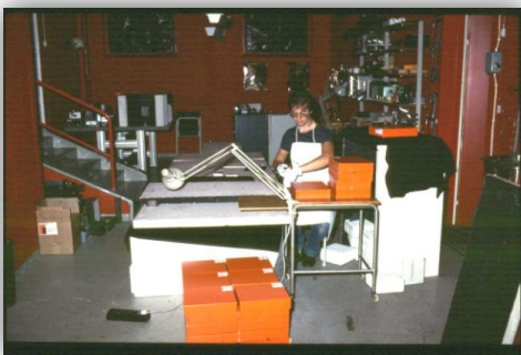
Lennart Svensson was recording all the holograms in the setup on the laboratory floor (200 plates/day). Note the Styrofoam block surrounding the setup to prevent air turbulence during the recording
