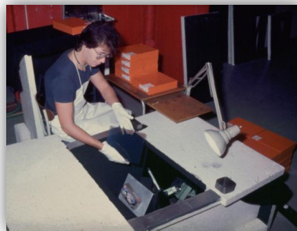
Lennart Svensson was recording all the holograms in the setup on the laboratory floor (200 plates/day). Note the Styrofoam block surrounding the setup to prevent air turbulence during the recording
