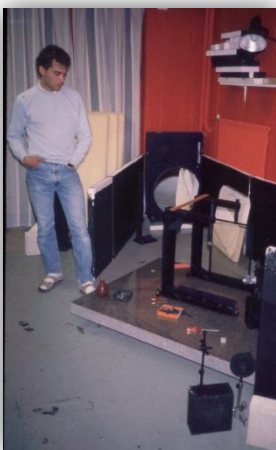
Jonny Gustafsson next to the transfer setup on the floor in the laboratory. Note the Styrofoam blocks to prevent air turbulence during the copy recording
