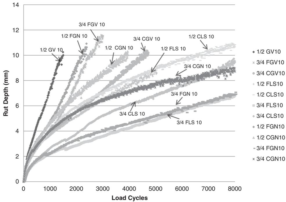
FIGURE 3 APA results for mixtures containing 10% natural sand.
