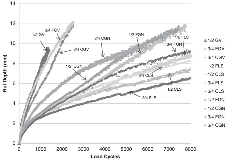
FIGURE 2 APA results for mixtures without natural sand.
