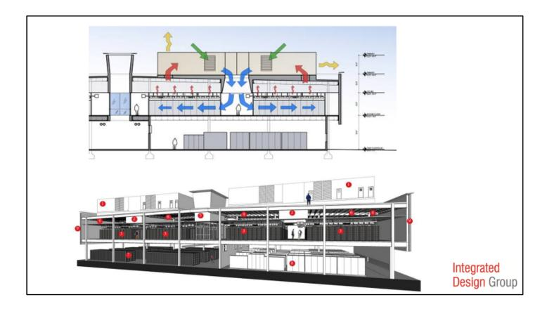
• Large openings and pathways for air flow to enhance natural ventilation and minimize fan power.
